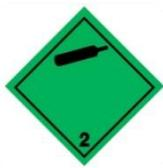
**LN<sub>2</sub> is inert, colorless, odorless, non-corrosive, non-flammable, tasteless, extremely cold, and has no warning properties. Special care must be taken by personnel who handle or work in areas where LN<sub>2</sub> is used. Nitrogen is not toxic, but it acts as a asphyxiant at high concentrations.**
