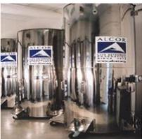
**Cryogenic Storage Tanks:** Typically includes a tank, a vaporizer, and a pressure control manifold. Cryogenic storage tanks may be spherical or cylindrical in shape. Their sizes range from 500-420,000 gallons. They are powder and vacuum insulated [4].
