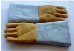
**Cryogenic gloves:** Wear cryogenic gloves for the spillage risk of cryogenics. Use large size to allow quick removal.
