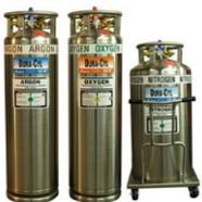
**Cryogenic Liquid Cylinder:** Cryogenic liquid cylinders are, Insulated, vacuum jacketed pressure vessels. They operate up to 350 psi and have capacities between 80-450 L. Product may be withdrawn as a gas by passing through an internal vaporizer or as a liquid under its own vapor pressure. They become equipped with safety relief valves and rupture discs. This protects from pressure
